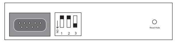
Dip Switch 3 is in the Down/ON position. Use this setting when connecting the RCV-5000 to a host PC for programming. Dip 3 must be turned ON (Down) before the RCV-5000 program auto-scan will recognize the RCV-5000. Once programming is complete, move Dip 3 to the UP/OFF position.
