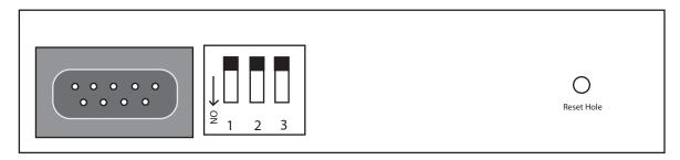
Use this Dip switch setting (all dip switches in UP/OFF Position.
